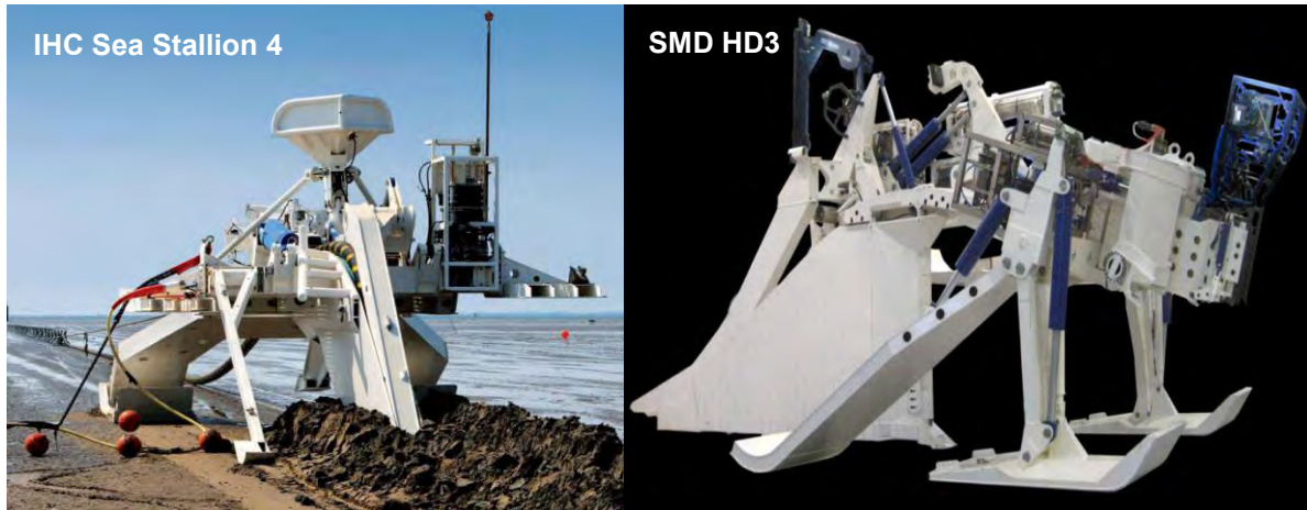
Figure 54 Example Power Cable Ploughs
