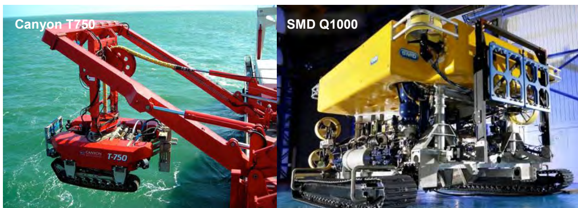
Figure 55 Example Power Cable Jetting ROVs
